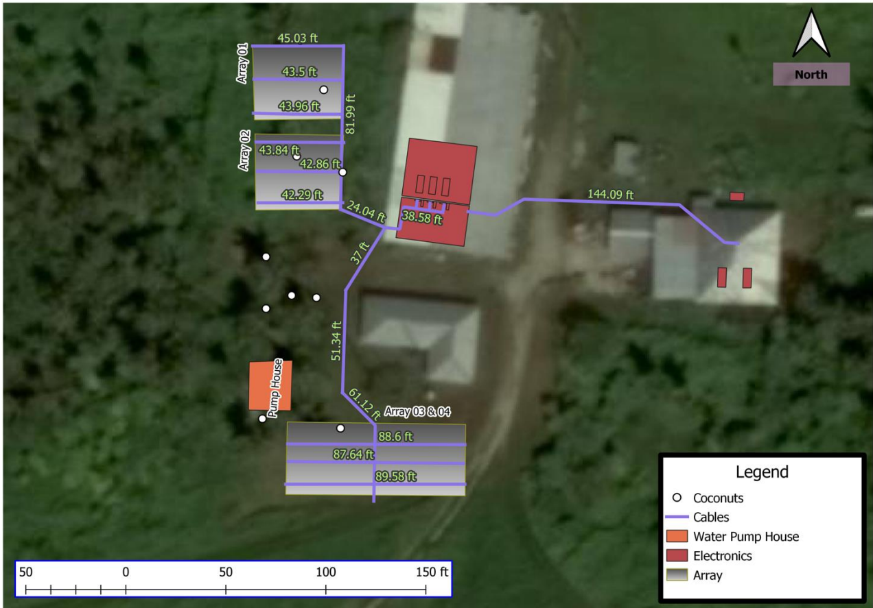
Photo2 – Ulithi Falalop 60kWp Layout: 30kWp + (2 x 15) kWp
