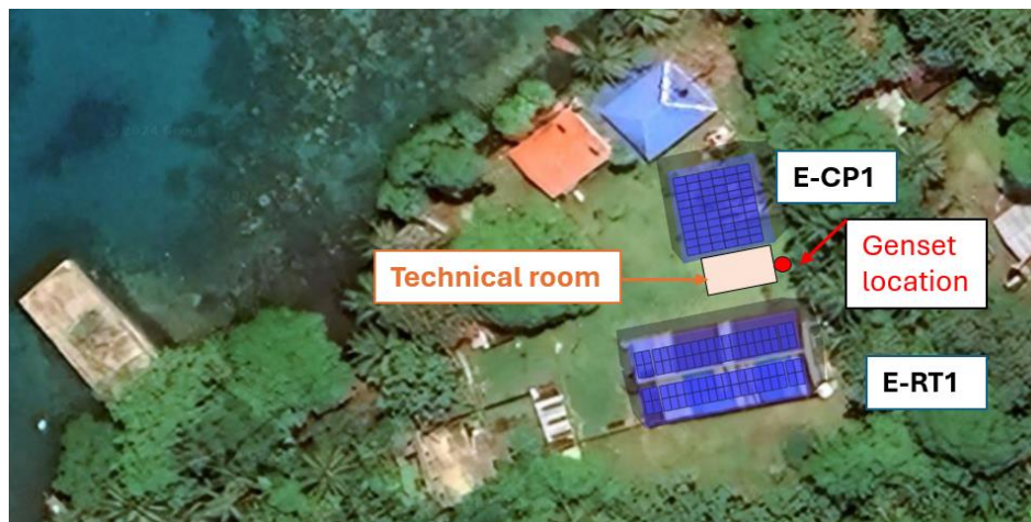
Figure 34. Option 2: Satellite view of the space available for technical room in Etten
