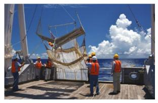
Trawl nets used to collect micronekton (image: Élodie Vourey).
