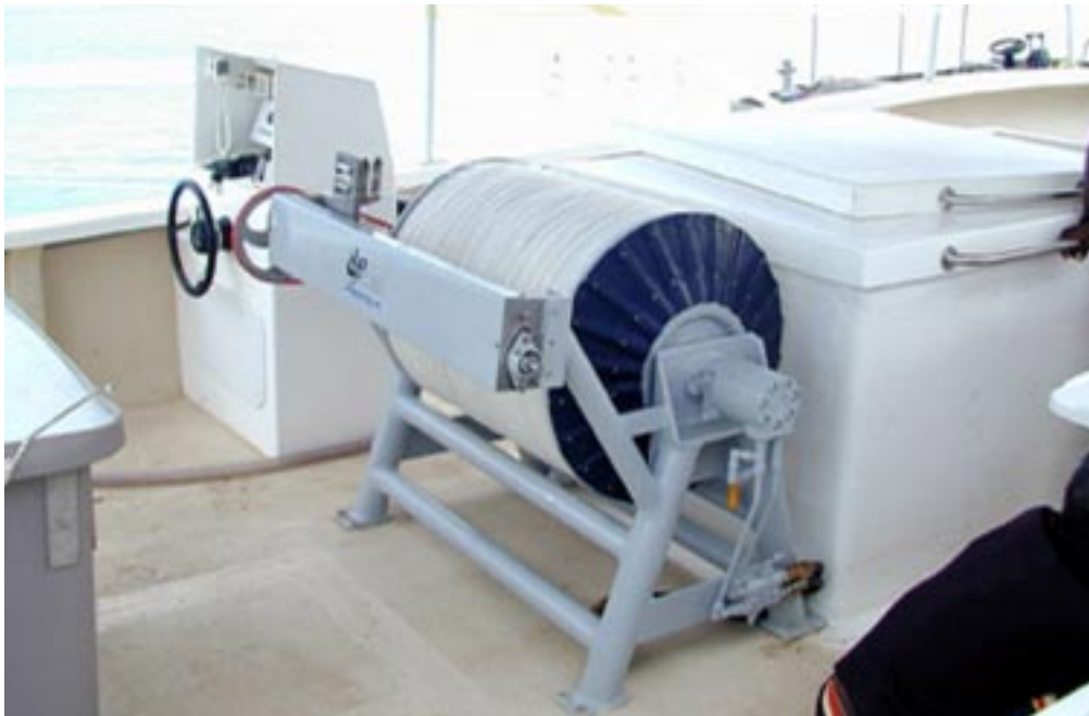
An 11 m longliner, showing placement of the Lindgren-Pitman 24" x 27" longline reel, and the control station. The insulated fish box is just forward of the reel and a branchline bin is secured in chocks just aft of the reel.
