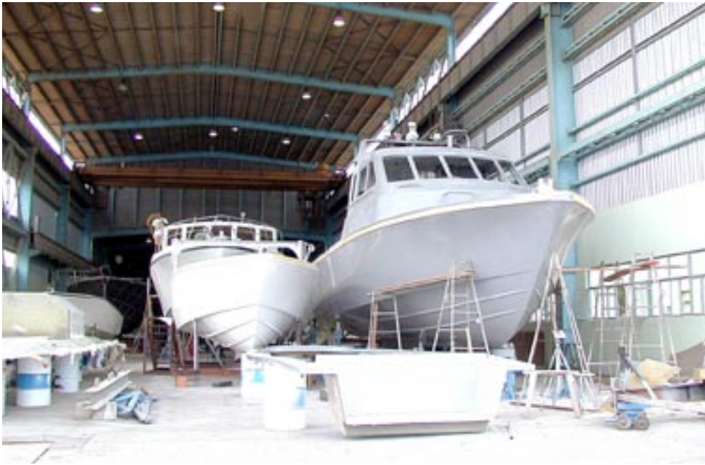
The boathouse at Harena boatyard showing several vessels in the works: an 11 m fishing boat and a 17 m patrol boat in the foreground, and an 18 m longliner behind the 11 m
