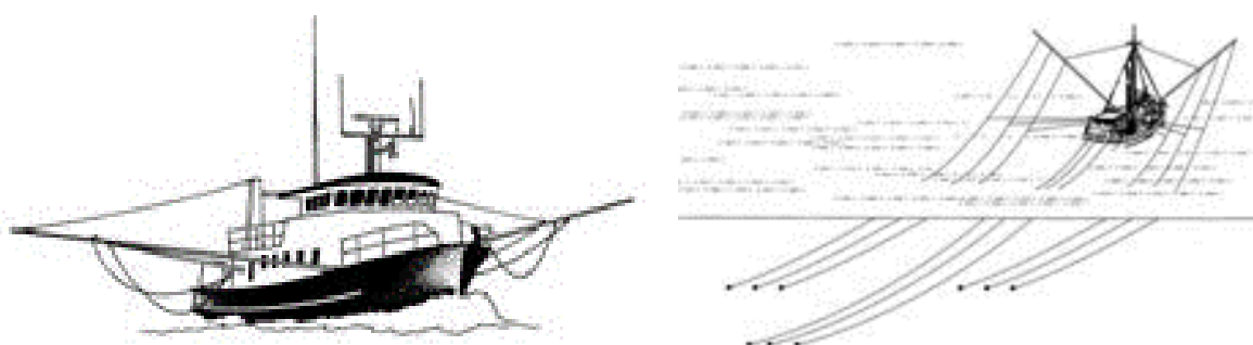
Figure 3.4 Troll vessel and gear
