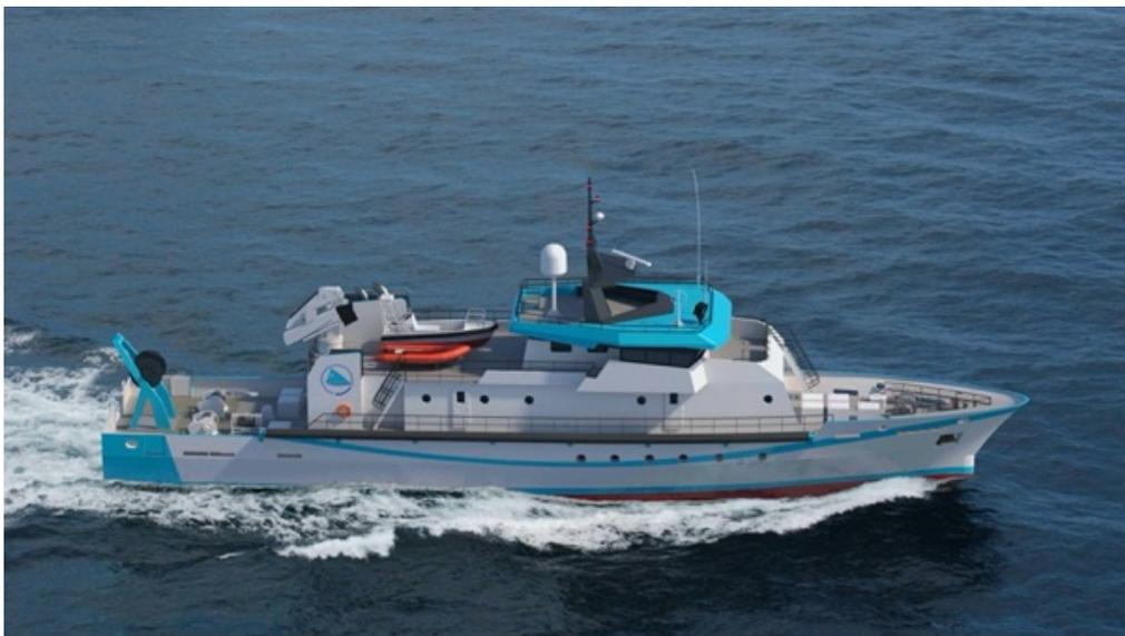
*43-meter hull, diesel-electric propulsion; this adaptable platform's main objective will be directed to collect data on tuna species and their environment. Facilitating SPC members' capacity building will also be reflected in the vessel design.*
