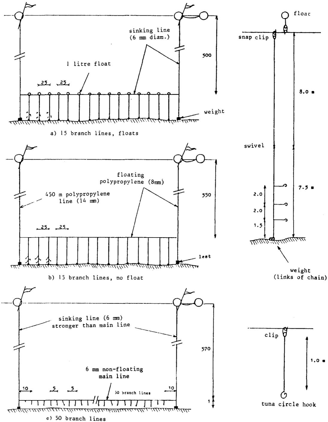
Fig. 6 - Experimental bottom longline used during the exploratory survey of R.V. VAUBAN. Different gear arrangements a,b, c used, (from Fourmanoir, 1980, and Fourmanoir and Chabanne, 1980).
