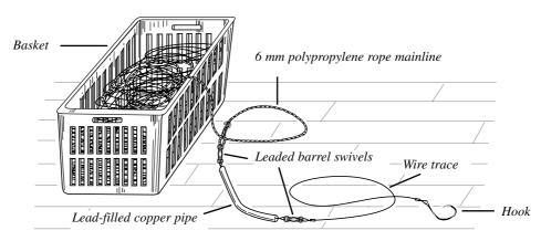
Figure 12: Ika-shibi fishing line arrangement
