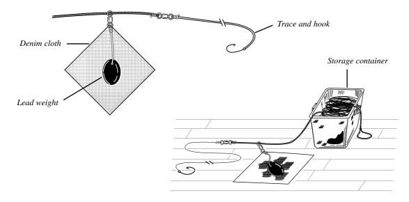
Figure 15: Palu-ahi fishing gear arrangement
