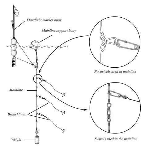
Figure 9: Two types of attachment points for connecting branchlines to the mainline
