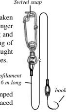
Figure 10: Branchline construction
