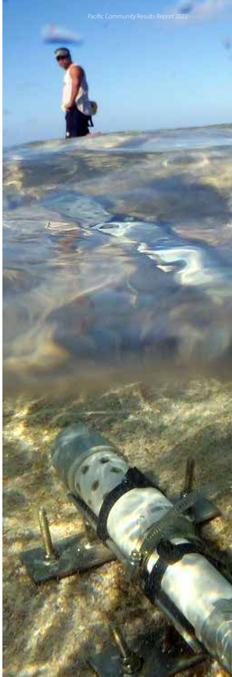
Temporary tide gauges/pressure sensors are deployed and used by the Oceans Monitoring and Predictions Team in the GEM Division to measure tides and waves.
