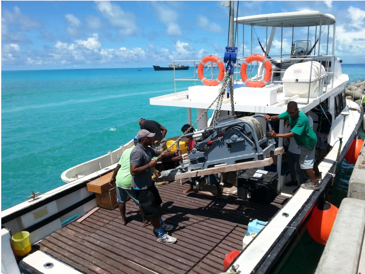
Figure 30: Setting the winch system on the survey boat. A dual frequency echo sounder, purchased by the Korean Research Institute of Ships and Ocean Engineering, was mounted on the starboard side of the boat.
