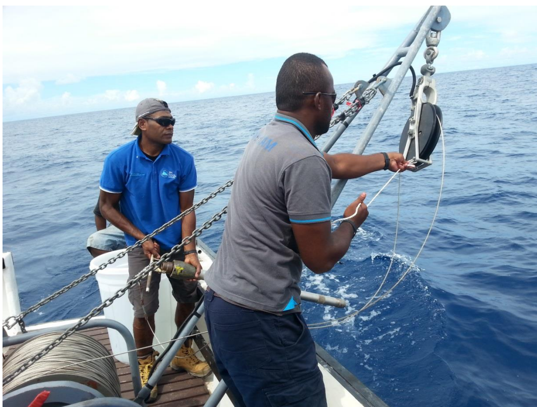
Figure 32: Geoscience Division technical staff deploying the gravity corer to depths of ~1,000 m. The launch was controlled using the winch motor break and released in free fall when the corer was ~30 m above the sea bed.
