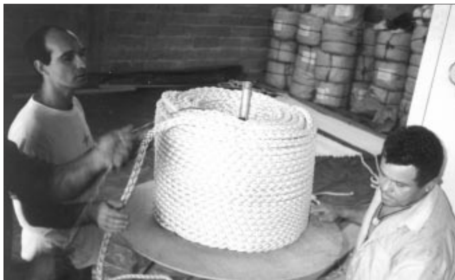
Figure 14: Turntable arrangement used for uncoiling ropes for the FAD mooring
