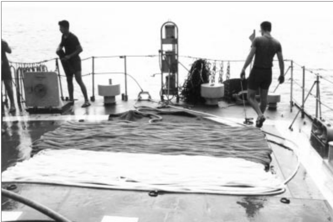
Figure 12: Mooring line flaked on back deck with ends going over the stern through a fairlead
