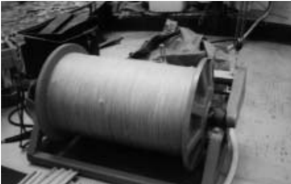
Figure 11: Mainline reel about 75 per cent full of 3.0 mm monofilament
