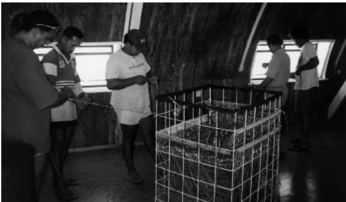
Figure 27: Making up new branchlines from 3.0 mm tarred red polyester line, with leaded swivel and wire trace
