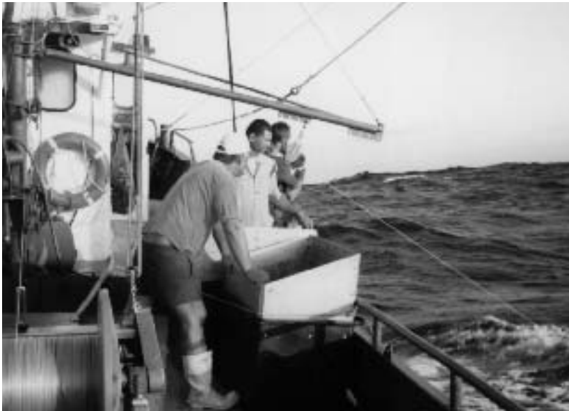
Figure 29: Incorrect method of removing snaps from the mainline during hauling
