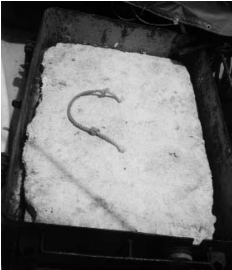
Figure 10: Ill-fitting make-shift plug for fish hold
