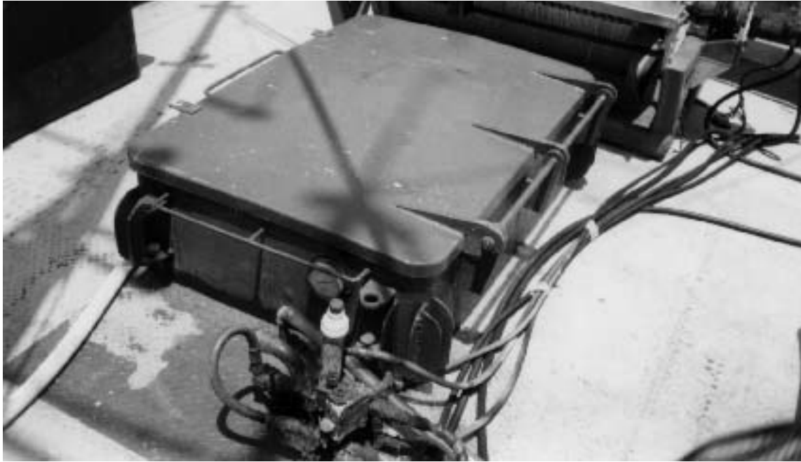
Figure 9: Blanked-off pipes and hydraulic hoses forward of fish-hold hatch
