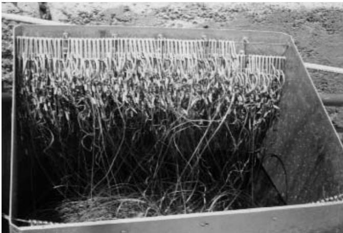
Figure 16: Branchline bin with branchlines—some in poor condition
