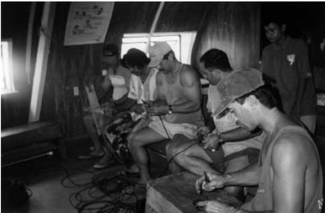
Figure 34: Workshop participants splicing 6.4 mm tarred Kuralon to make a vertical longline
