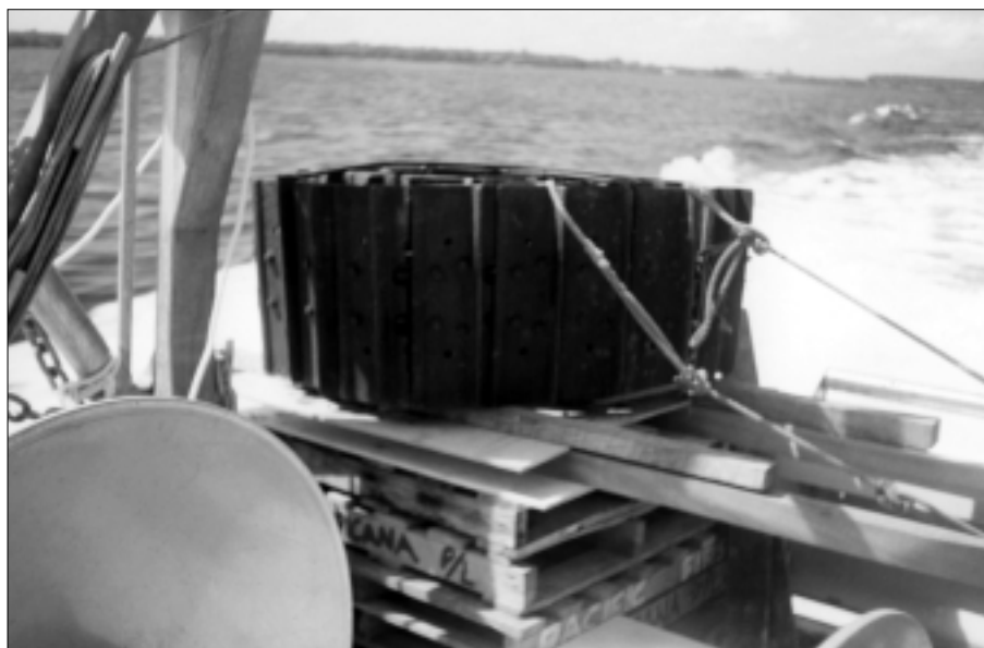
Figure 20: Bulldozer track on platform ready for FAD deployment
