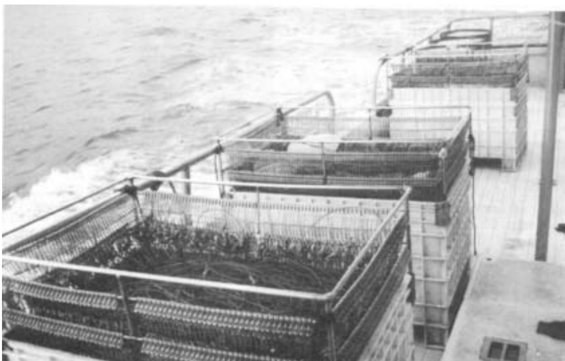
Figure 11: The new tarred red polyester branchlines stored in the three bins
