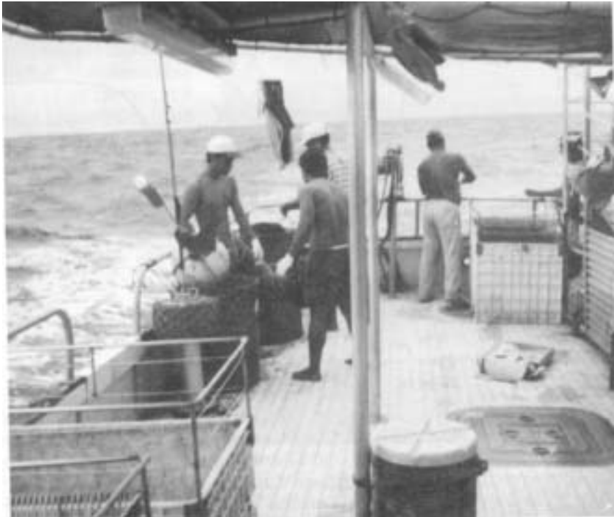
Figure 12: Setting the tuna longline using the line shooter on NFC Waab— branchlines being set off the port side
