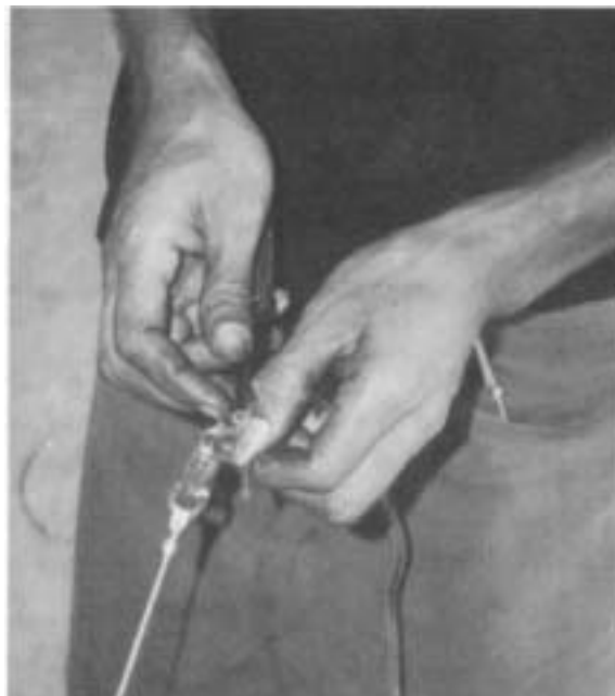
Figure 10: Using a Swedish fid to tuck the end of the tarred red polyester line back into the lay of the line
