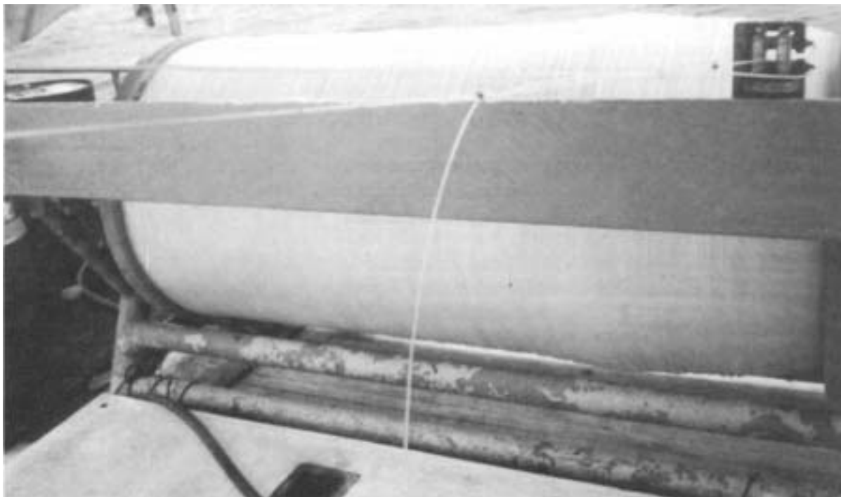
Figure 6: LP reel with new monofilament mainline installed
