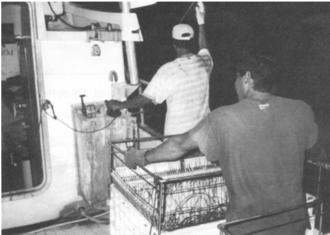
Figure 15: Roller man operating the controls for the reel, throttle, and steering while unsnapping the branchlines from the mainline
