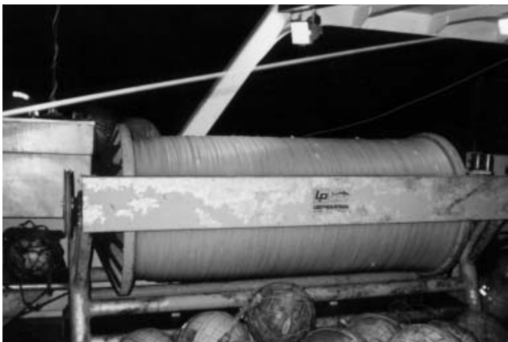
Figure 8: Lindgren-Pitman monofilament reel with reduced amount of mainline
