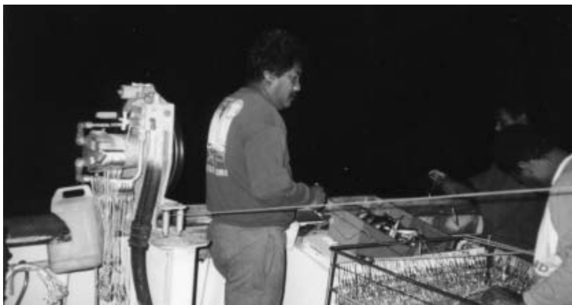
Figure 10: Crewman taking branchlines from bin to pass the clip to the snapper and the hook to the baiter
