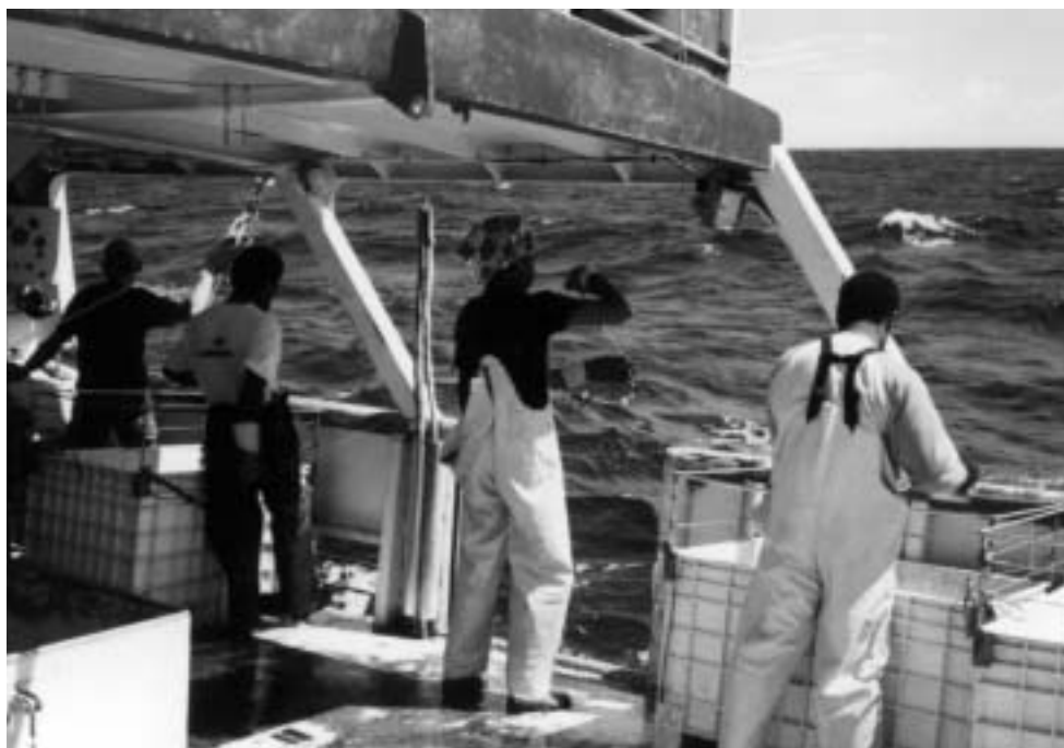
Figure 9: Crewman standing in front of gate to pass branchlines around stanchions
