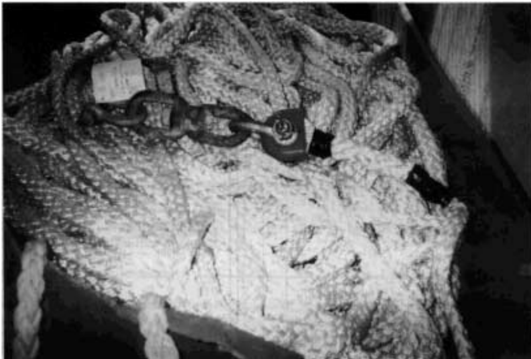
Figure 13: Rope-to-hardware connection, showing an eye splice protected with nylite connector and black waterproof tape
