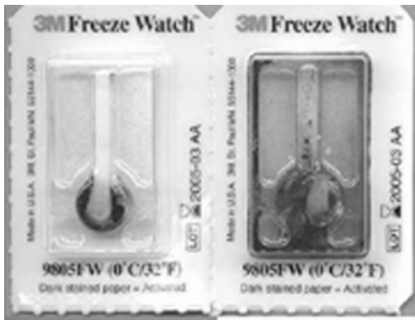
Figure 4. Freeze Watch indicators. Left- Normal indicator, not frozen, Right- Activated (burst) after exposure to temperatures below 0°C
