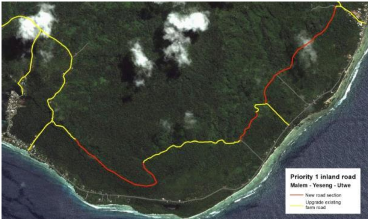
Figure 4-3: Indicative inland road between Utwe and Malem showing the requirements of new and upgraded sections of road.
