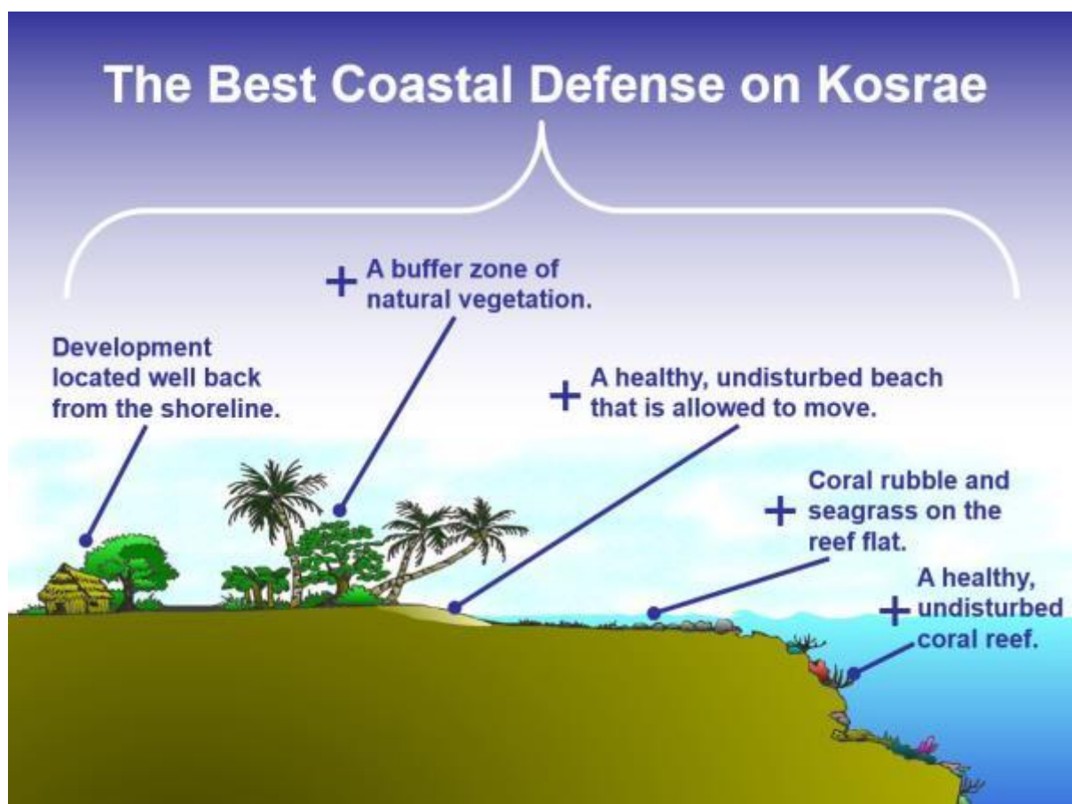
Figure 3-1: The best coastal defence on Kosrae. Awareness poster developed in 1999 by the Development Review Commission (now KIRMA).
