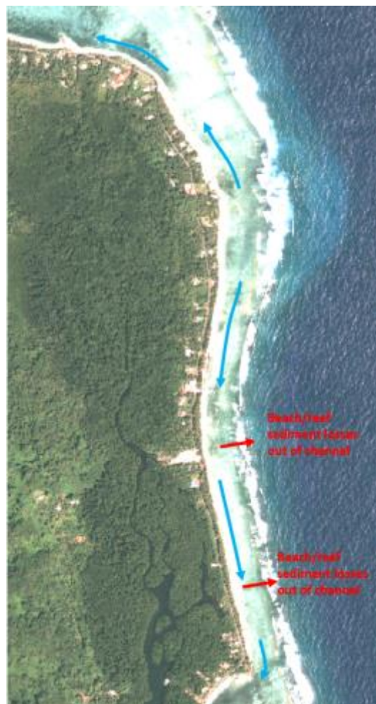
Figure B-10: Key sediment sources, longshore transport processes, and sediment losses along the Pukusruk shoreline.
