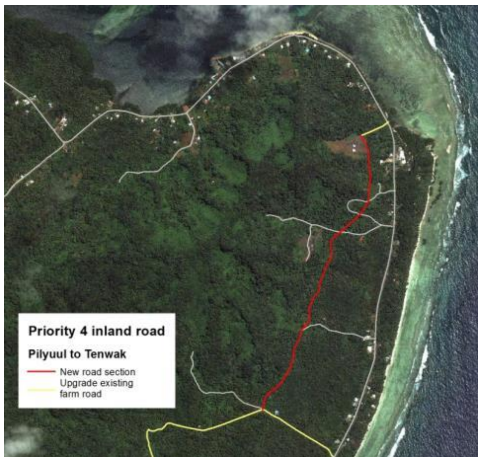
Figure 4-7: Inland road section between Pilyuul and Tenwak.
