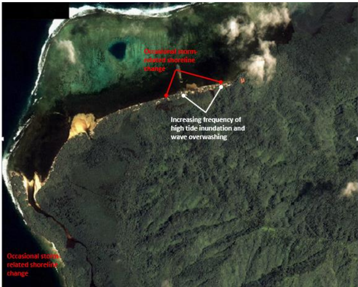
Figure 2-5: Potential areas of inundation and erosion concern in Walung over the next one to two generations.
