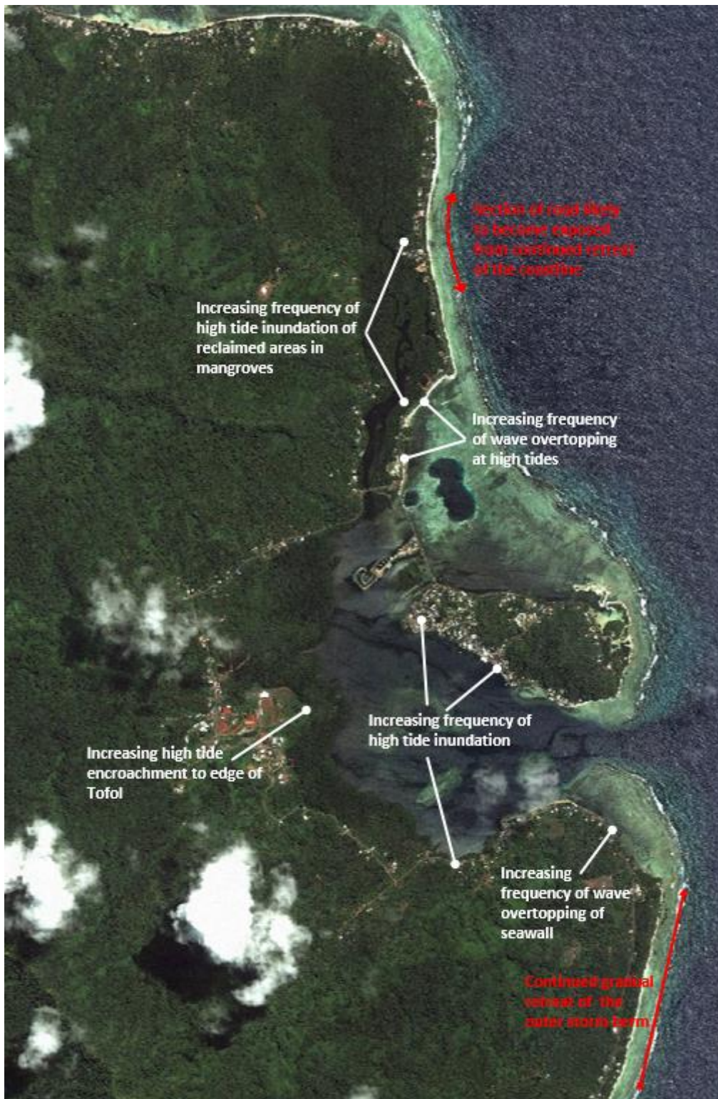
Figure 2-1: Potential areas of inundation and erosion concern in Lelu Municipality over the next one to two generations.
