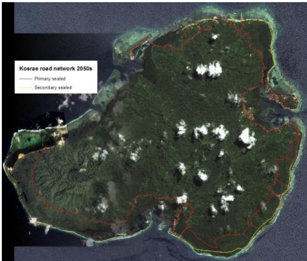
Figure 4-1: Potential primary and secondary sealed road network on Kosrae by the 2050s. Note: Parts of the secondary road network (current coastal road) may become impassable due to ongoing shoreline change and breaching.
