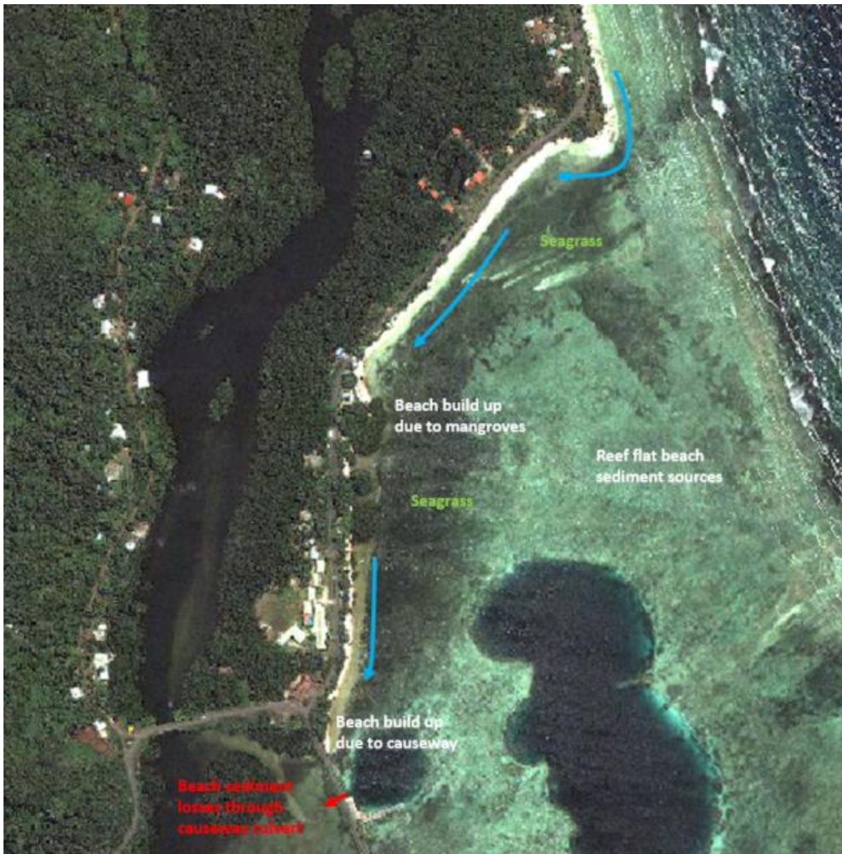
Figure B-5: Key sediment sources, longshore transport processes, and sediment losses along the Putukte to Finpukal shoreline.
