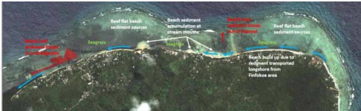
Figure B-3: Key sediment sources, longshore transport processes, and sediment losses along the Tafunsak shoreline.
