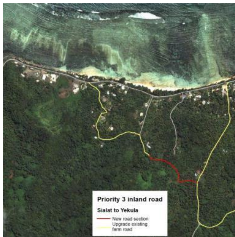
Figure 4-5: Inland road section between Sialat and Yekula.
