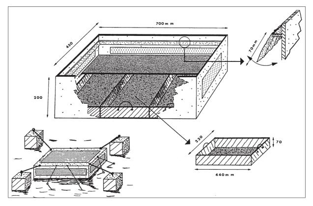
Figure 1: Design of the modified polypropylene boxes used during the field experiments
