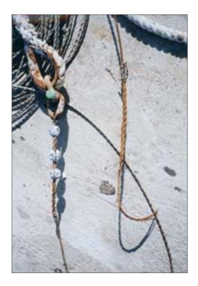
9.0 mm galvanised wire cable showing splices, one parted
