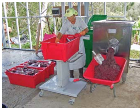
Figure 4. Grinding tuna waste for the production of fish silage (fertiliser) (image: BioAgri-NC).
