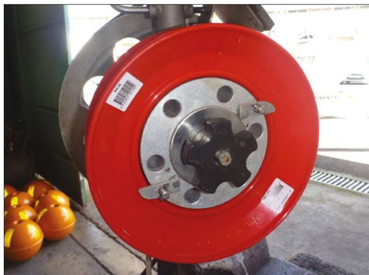
Figure 5. A plastic spool fitted onto the coupling and locked in (image: Mainui Tanetooa).
