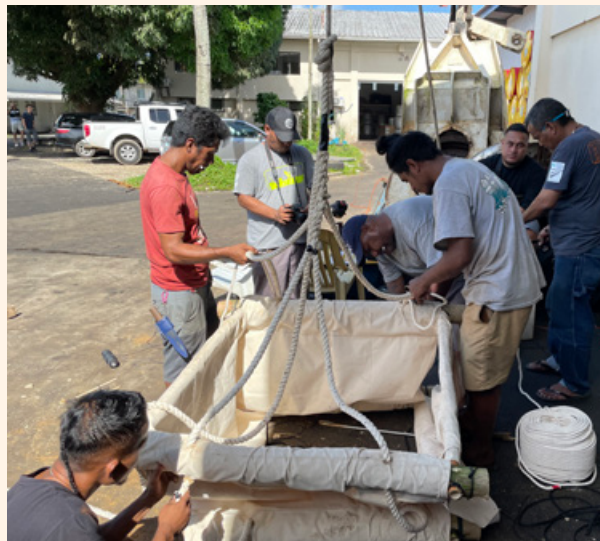
Attaching the cotton ropes to the drogue. ©William Sokimi, SPC
