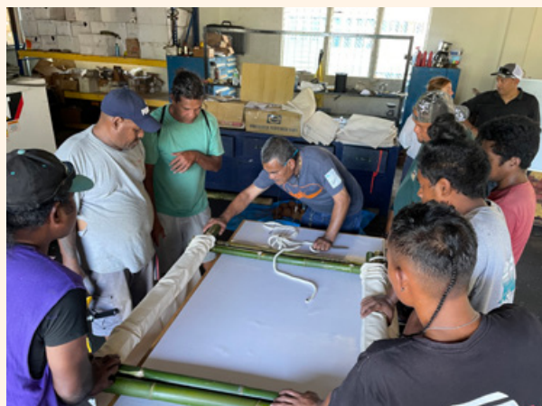
Building the submerged raft with bamboo and cotton canvas. ©William Sokimi, SPC
