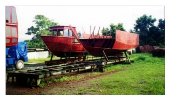
Figure 2: Ten-metre deep-bottom fishing vessels under construction
