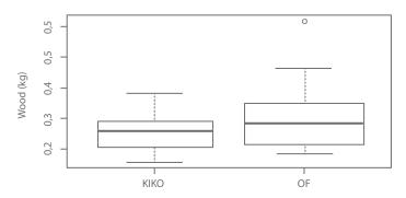
**Figure 7.** Wood (kg) needed to boil one litre of water (kiko stove versus open fire, n = 30).
