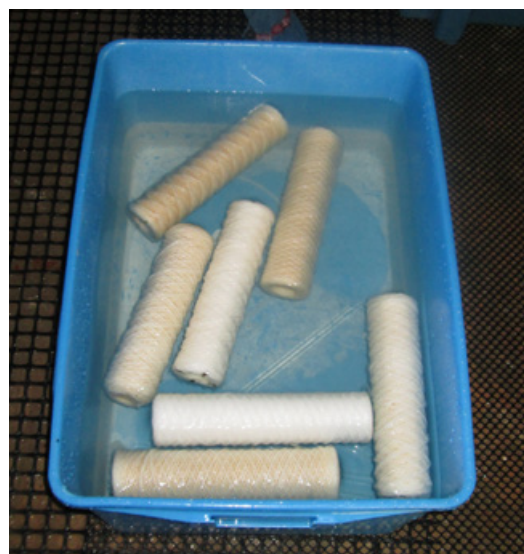
Disinfection of cartridge filters
