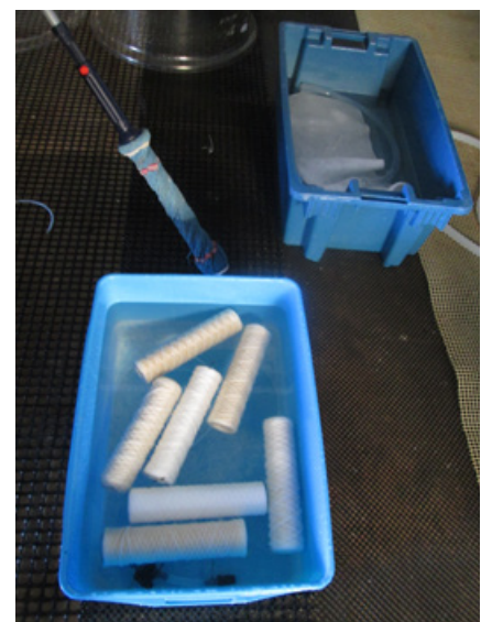
Disinfection of cartridge filters
