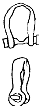
Badly worn hardware components
