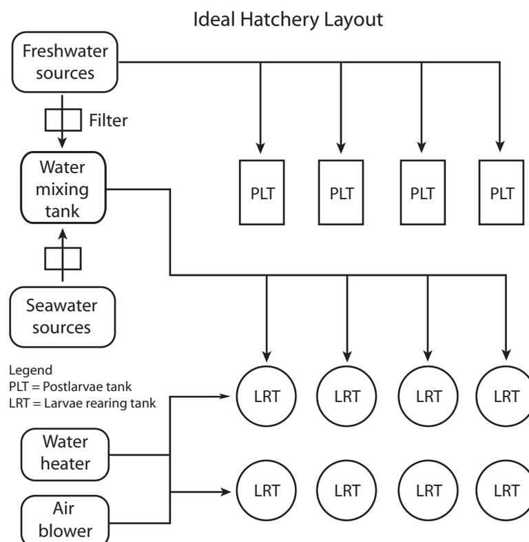
Fig. 5. Ideal layout of a semi-commercial/back-yard freshwater prawn hatchery
