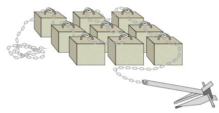
Figure 28. Diagrammatic representation on connecting multiple small blocks with galvanised chain.
