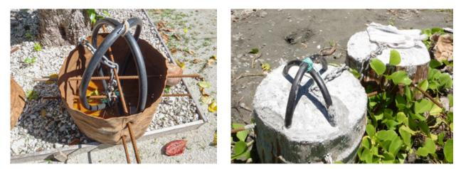
Image 3. Dual drum anchor showing the internal set-up (left) and prior to being deployed (right).
