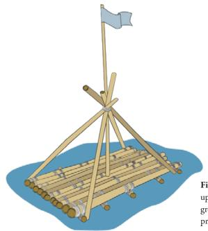
**Figure 5.** Large bamboo rafts are often used for the upper floatation of bamboo FADs, which can place greater stress on the mooring system and result in premature loss.
