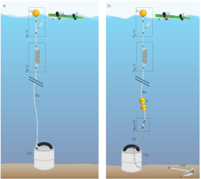
**Figure 4.** Bamboo FAD design showing: a) the basic version suitable for lagoons and bays; and b) the advanced version with additional anchor capacity being more suitable for nearshore environments. More detail on the components in each of the boxed inserts can be found in section 4.
