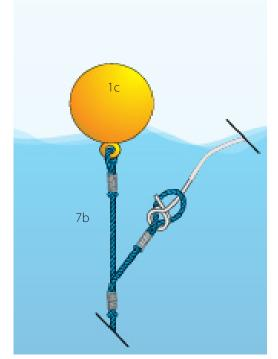
**Figure 14.** Diagram showing the detachable loop on the upper floatation for the bamboo FAD.
