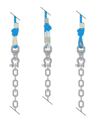
Figure 29. Anchor to main line rope connection.
