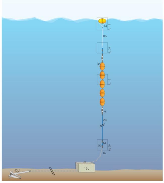
**Figure 7.** Subsurface FAD design showing the temporary surface marker to aid fishers to locate the FAD initially. More detail on the components in each of the boxed inserts can be found in section 4.
