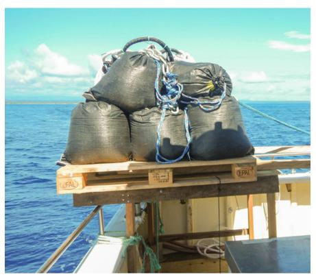
Image 7. Anchor constructed from sandbags.
