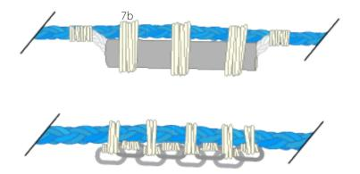
**Figure 22.** Diagram showing two counterweight options – cement tube (top) and galvanised chain (bottom) – and how they are rigged to the mooring line.
