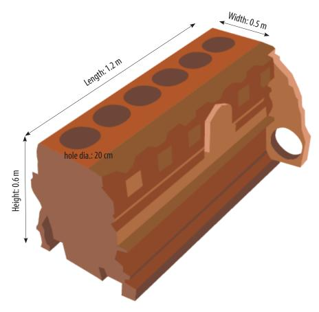
Figure 27. Example of calculating the volume of a recycled steel engine block anchor.
