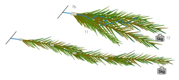
**Figure 21.** Diagram showing streamlined bamboo aggregators connected end-to-end in series (bottom) and bunched (top).
