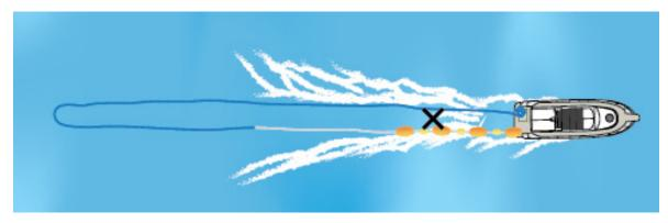
Figure 33. Sub-surface and lizard FAD deployment technique. The cross (X) represents the intended final anchor location.
