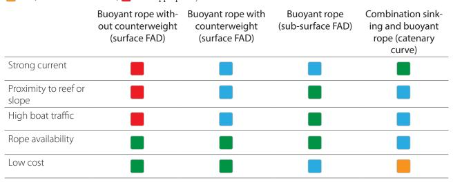
**Table 5.** Optimal FAD mooring system designs based on different parameters ( = optimal, = sub-optimal, = ok, but not recommended, = not appropriate).
