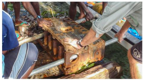
Image 6. Anchor constructed from a recycled engine block.
