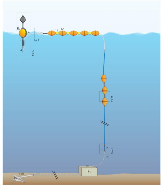
Figure 8. Lizard FAD design. More detail on the components in each of the boxed inserts can be found in section 4.
