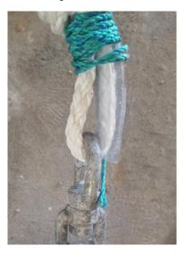
Image 1 shows a FAD that was poorly constructed. The FAD was in the water for less than one month before washing ashore. While the FAD was lost due to a different connection than the one pictured here, you can see that the whipping around the plastic tubing was not tight or long enough to hold the tubing in place. If other sections of this FAD did not break, eventually the tube would have cut the rope at this point.
