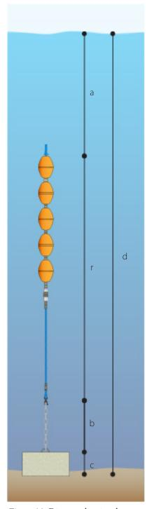
**Figure 23.** Diagram showing the components required for the calculation of subsurface main line rope length (a = floatation settling depth, b = chain length, c = block height, = deployment depth, r = main rope).
