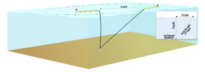
Figure 26. Diagram showing a FAD's scope.
