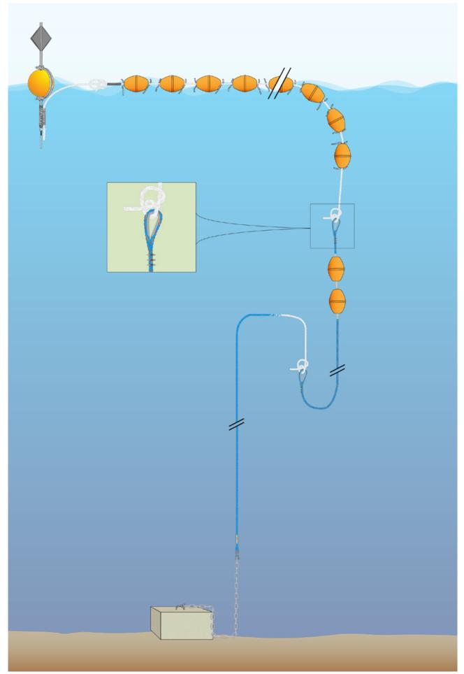
Figure 10. French Polynesia FAD design showing modifications.
