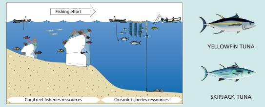
Installation of anchored fish aggregating devices (FADs) close to the coast (usually within 1–6 km from the shore at depths of 300–1000 m) is often the most effective way of providing small-scale coastal fishers with better access to the abundant skipjack and yellowfin tuna resources of the region (SPC 2012a, b).
