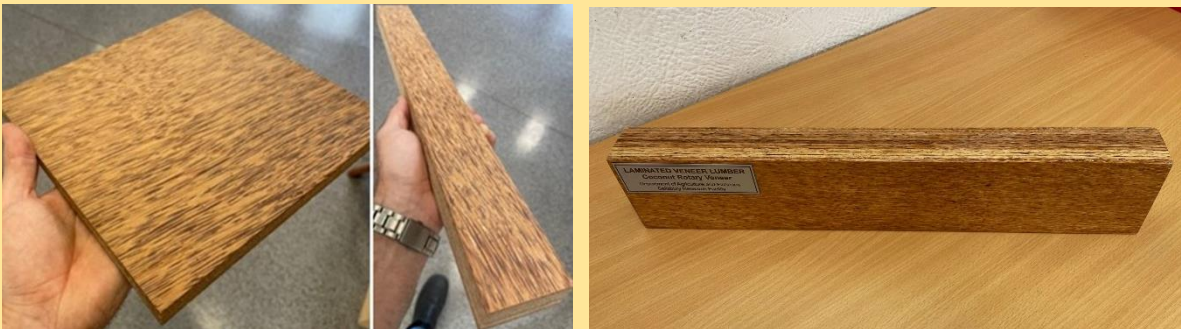
Fig. 4. Structural cocoveneer EWP: plywood (left) and LVL (right).
