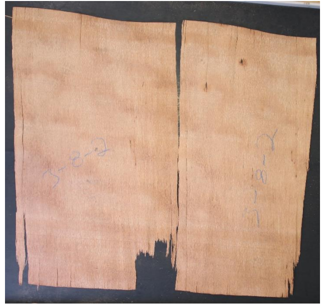
Figure 2 Example of Grade F coconut veneer, with severe tear-out (>75 mm) and defects beyond the minimum acceptable thresholds.
